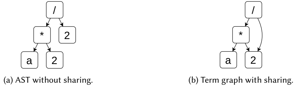
Figure 2.1: Different representations of the program (a * 2)/2 have different characteristics. The syntax tree is simpler (a), but the term graph is smaller since it captures sharing (b).
